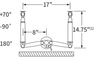
Shown desk mounted against wall with 16" wide monitors. Achieve additional depth with Grommet Mount further in on worksurface.
